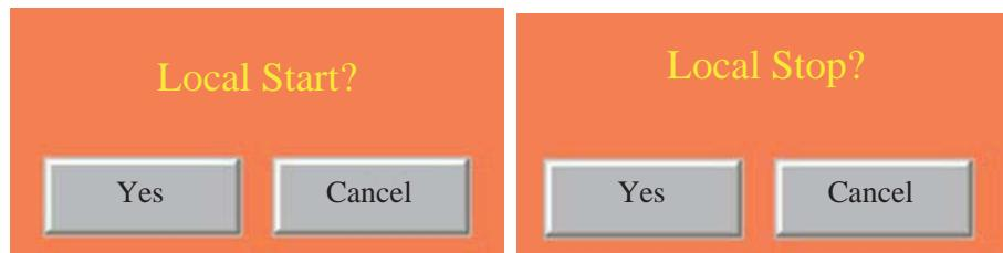
Local Stop: to stop the system by clicking the stop button on the HMI or on the door. The HMI pops up a prompt of stop confirmation, as shown in the above figure.
